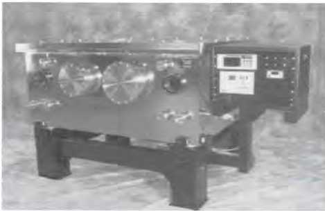
GPR, Inc.'s semiconductor chamber.
